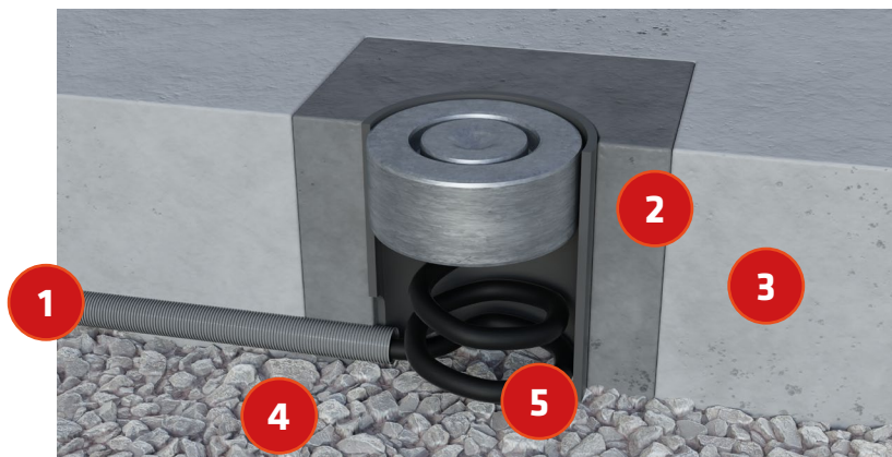
Example of installation of a temperature and moisture sensor in a pavement
